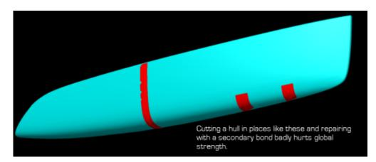
vinyester resin only achieved 66% of the tensile strength of the surrounding laminate. The study was not funded for the testing of epoxy resin but it was expected that epoxy will perform as well or slightly better than a toughened vinylester.
